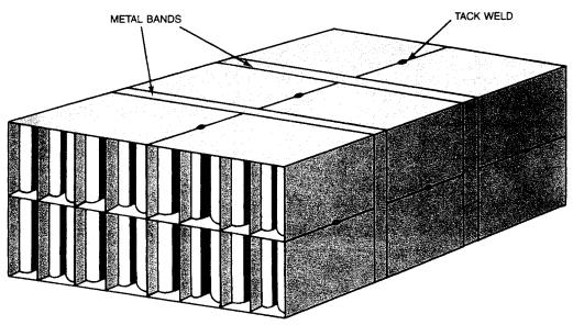
Assembly — Modules should be banded together with at least two metal straps or steel frames around entire bank. Three or four tack welds along the length of each adjoining surface should be made to provide structural rigidity.
