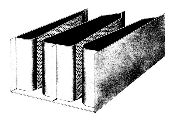
Outer casings are 22 gauge galvanized steel. All external seams are lockformed and filled with mastic or continuously welded, and are airtight up to 8" water gauge pressure differential. Casings are stiffened to prevent deformation when tested at 8" pressure differential, and stiffeners prohibit audible vibration during normal operation of air handling system.
